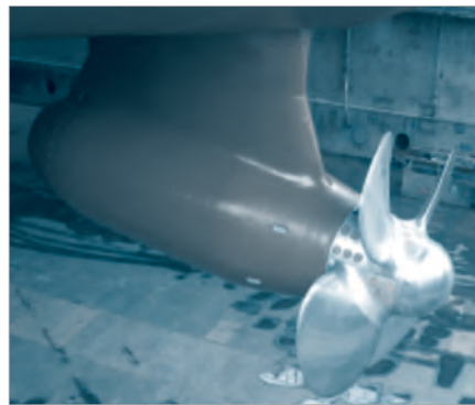
Figure IV.12 Azimuth thruster installed on an ice-going cargo ship
