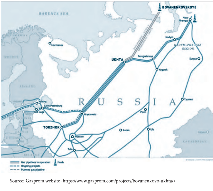
Figure IV.4 Bovanenkovo-Ukhta trunk line system
